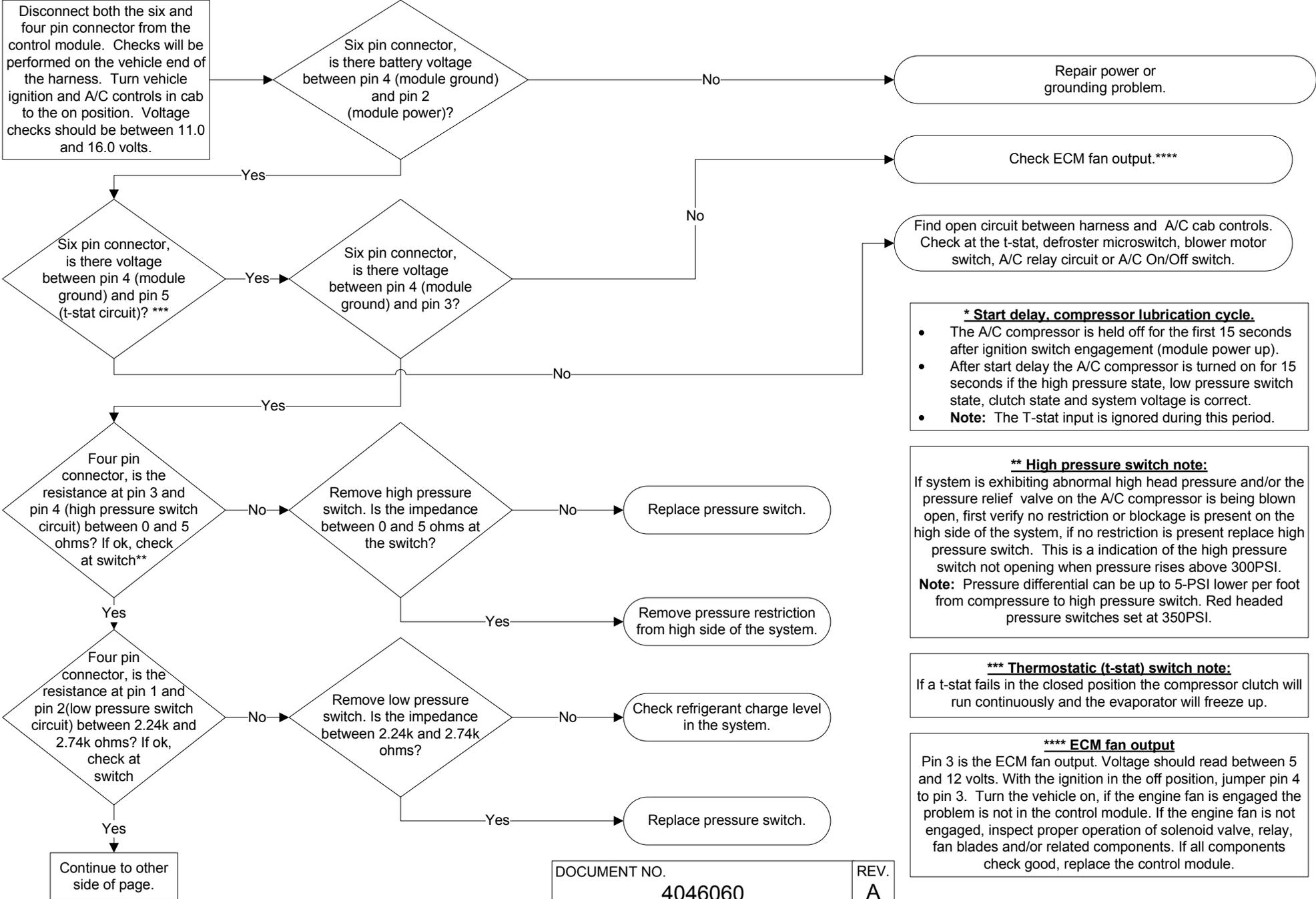
**\* Start delay, compressor lubrication cycle.**
