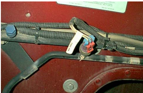
Figure 16: Pressure Switch Example
