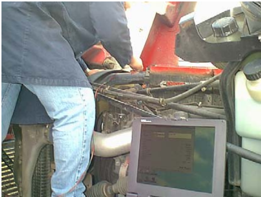
Figure 5: Data Logger and ACX Installation
