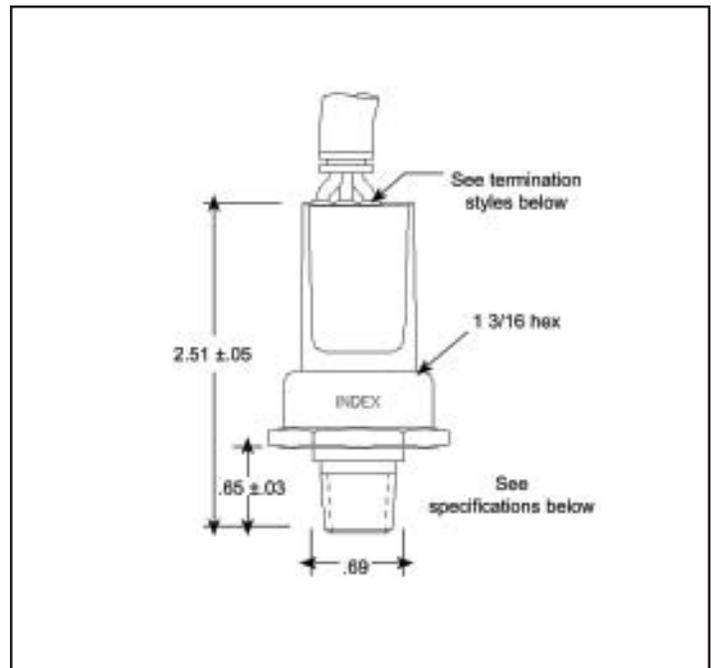
Index Heavy-Duty Pressure Switches are ideal for a variety of industrial vehicle & equipment uses, engine and transmission oil, fuel, air-conditioning systems, and custom applications.
